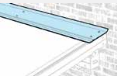
POWDER COATED INSULATED PANEL IN THE SAME COLOUR AS THE FRAME
